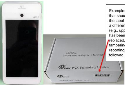
Example: This is official label that should be on the device. If the label has been relocated to a different place on the device (e.g., upper right) or if the label has been peeled off and replaced, this may indicate tampering and tampering reporting procedures should be followed.
